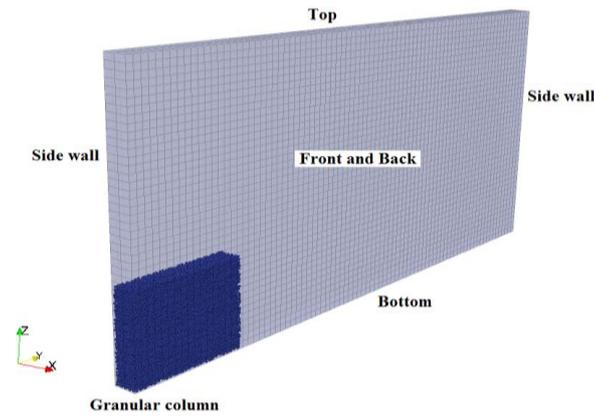
Figure 2 Simulation domain for submerged granular collapse
