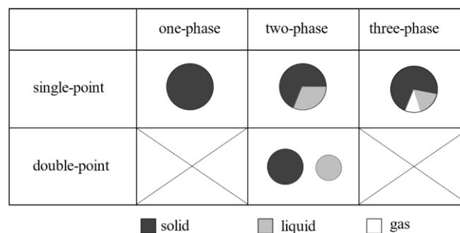
Figure 1 The different MPM formulation for geotechnical engineering (after Yerro & Rohe 2019)
