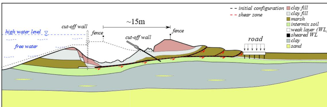
Figure 2 Schematic representation of a failed levee (modified from Seed et al. 2008)
