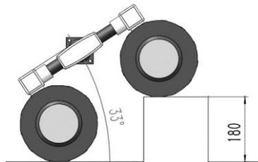
Figure 5 Maximum height of the obstacle can the wheel over
