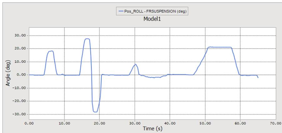
Figure 8 Swing angle of the suspension
