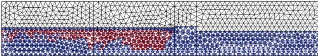
Figure 6 MPs where liquefaction occurred (in red colour)
