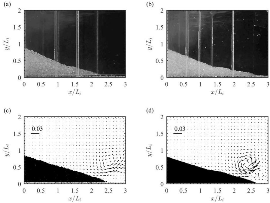
Figure 3 Final depositions from experiments and CFD-DEM simulations. (a) Experiment with  $L_i = 3$  cm; (b) Experiment with  $L_i = 5$  cm; (c) Simulation with  $L_i = 3$  cm; (d) Simulation with  $L_i = 5$  cm. The bars in (c) and (d) are scales for fluid velocity, which is normalized by a velocity scale,  $(gH_i)^{1/2}$
