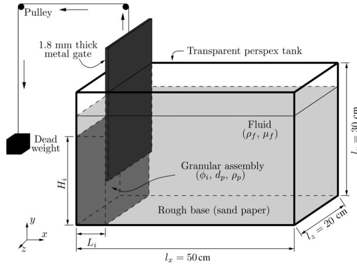
Figure 1 Experimental setup for the collapse of granular columns in water.  $L_i$  and  $H_i$  are the initial length and height of the granular columns
