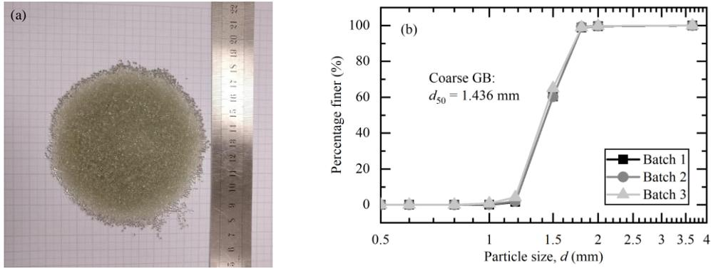
Figure 2 (a) GBs used to build the granular columns; (b) Particle size distribution curves of three individual batches from QICPIC analysis. The averaged  $d_{50}$  is 1.436 mm
