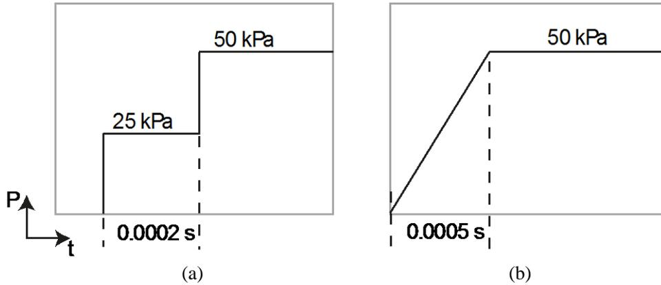
Figure 4 Load functions: (a) stepwise and (b) linear load functions
