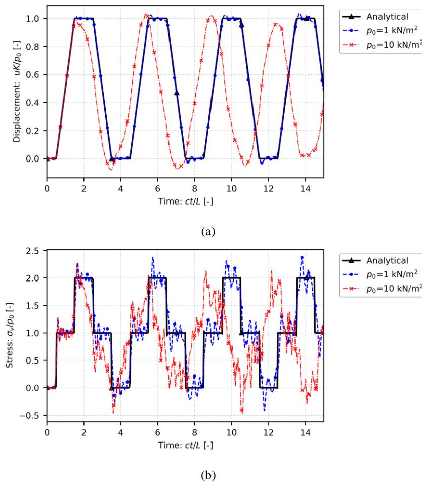
Figure 2 Comparison of the velocity for a point located on the solid column: (a) displacement and (b) stress of a point located at  $x = 0.5 L$ .
