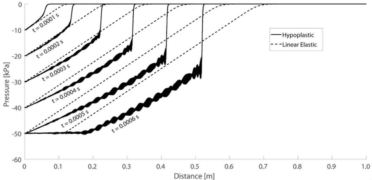
Figure 6 Linear elastic and hypoplastic solutions for linear loading.
