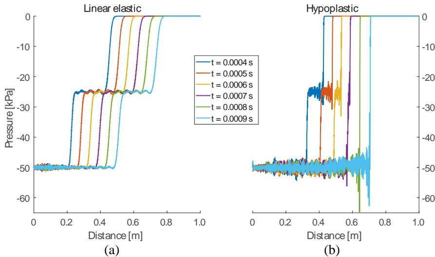
Figure 5 Solutions for stepwise loading with: (a) linear elastic and (b) hypoplastic material model
