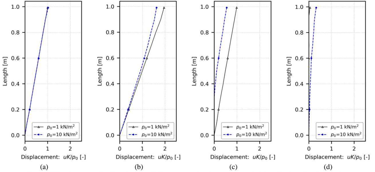
Figure 3 Displacements for the column at different normalised times: (a)  $t = 1$  (b)  $t = 2$  (c)  $t = 3$  and (d)  $t = 4$ .
