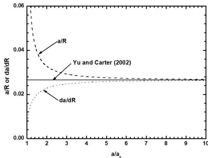
Figure 5 Variation of  $a/R$  and  $da/dR$  for a cylindrical cavity
