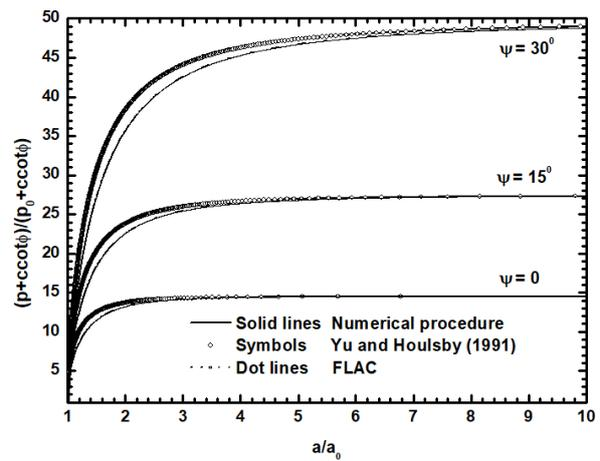
Figure 4 Pressure expansion curves for spherical cavities
