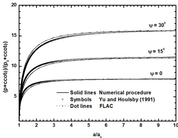
Figure 3 Pressure expansion curves for cylindrical cavities
