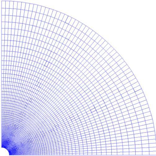
Figure 1 FLAC grid geometry for the model
