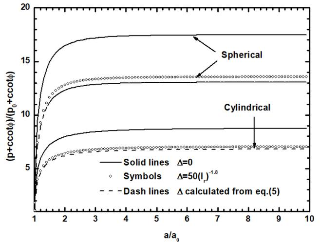
Figure 2 Pressure expansion curves for Vesic solutions
