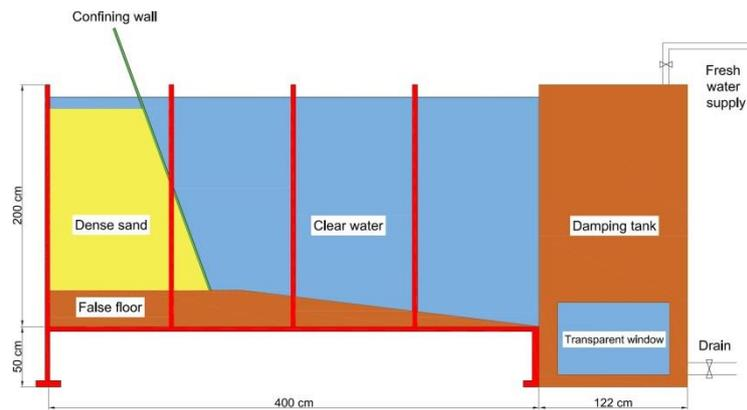
Figure 5 Side view of the experimental setup
