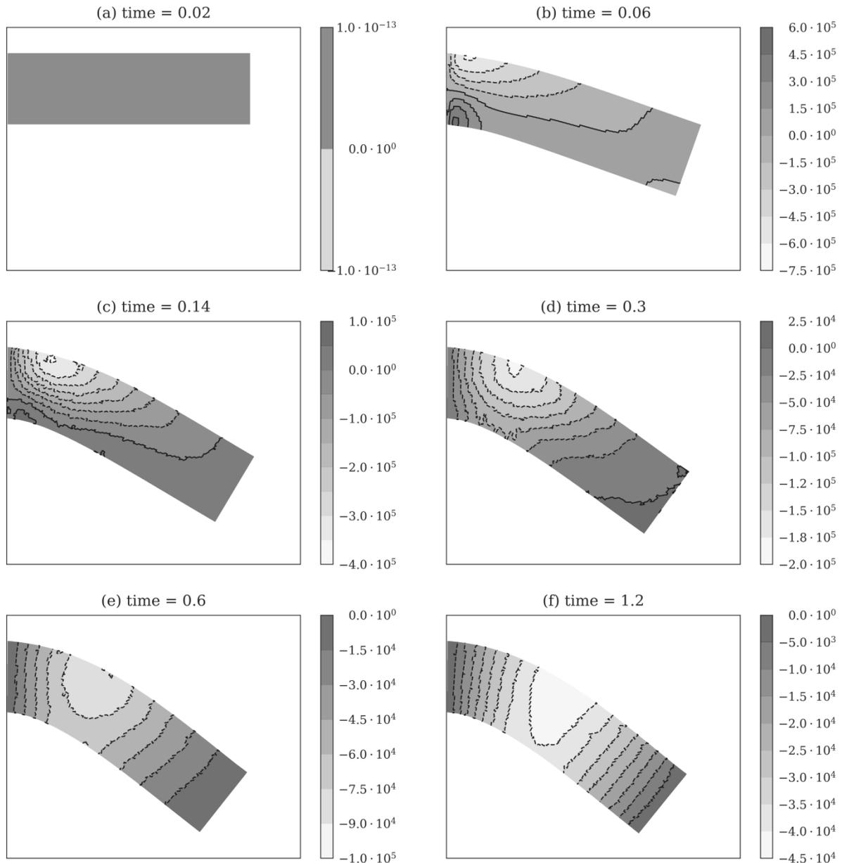
Figure 1 Material point pore pressure distribution in the poroelastic beam subject to a distributed load of  $q=54$  kPa. Pore pressures are in Pascal, with suction negative. Time is in seconds.
