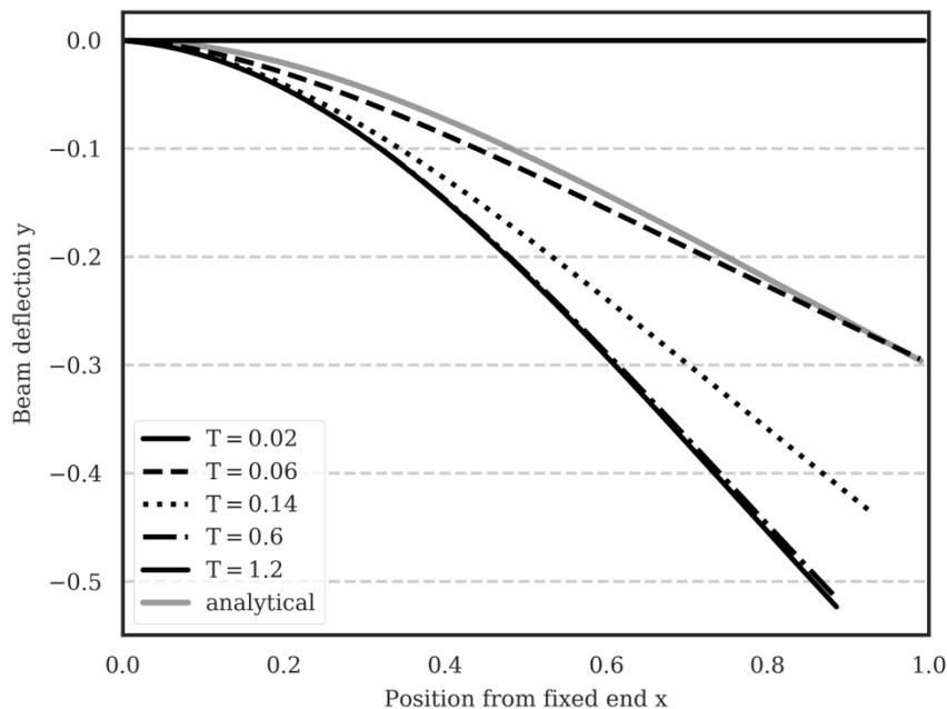
Figure 2 Deflection curves of the poroelastic beam at various simulation times. Time is in seconds, length is in metres.
