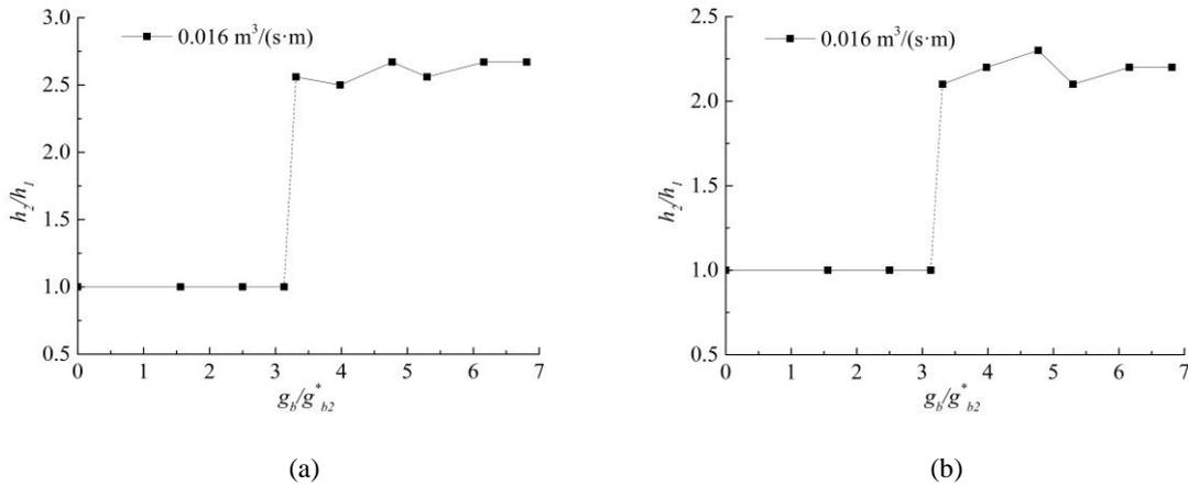
Figure 1 Water depth change over different slopes: (a) 5% slope channel; and (b) 1% slope channel
