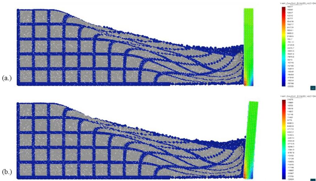
Figure 4 Deformed configuration of the soil-structure interaction tests of granular flow impacting (a) rigid and (b) flexible structure
