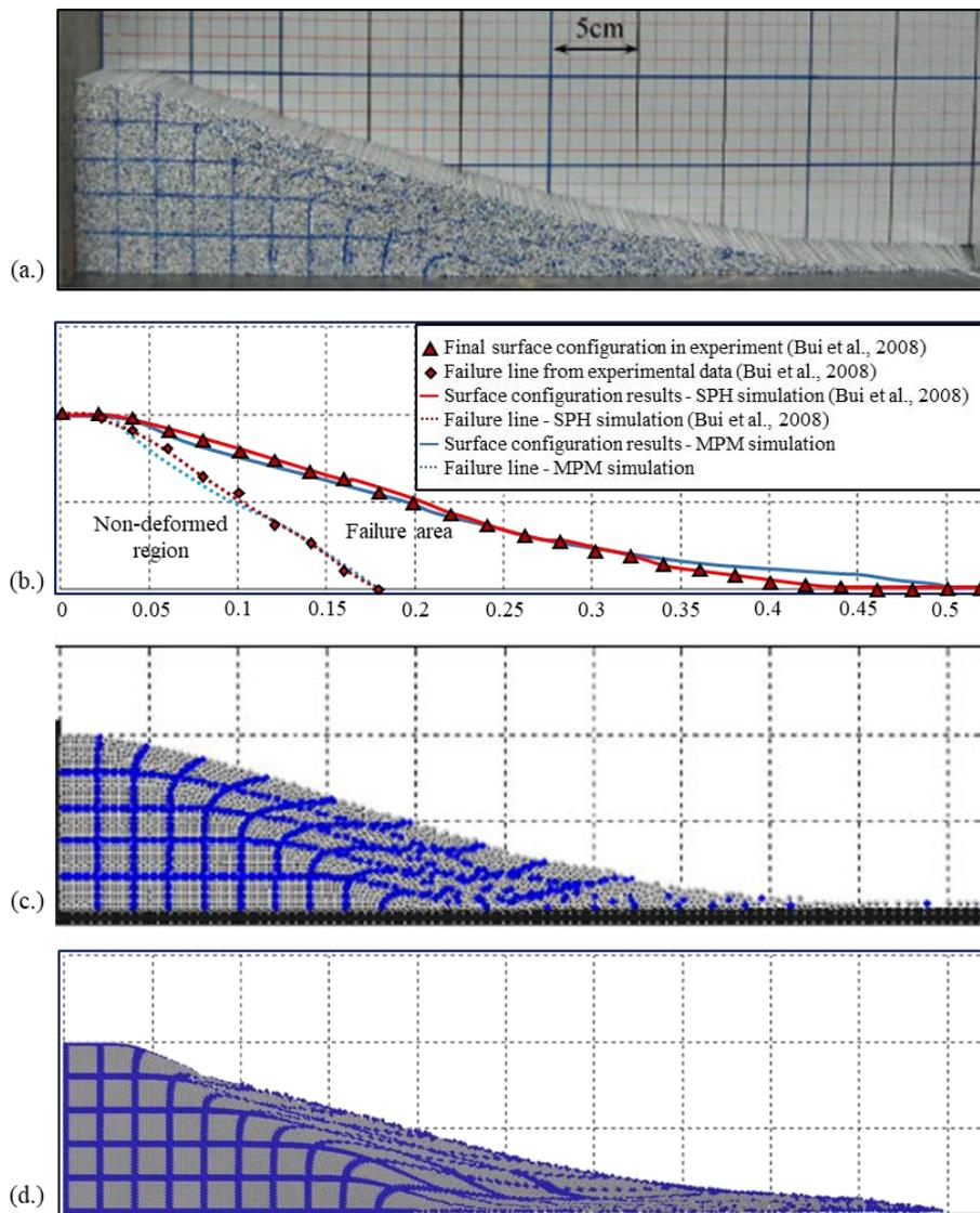
Figure 2 Granular flow validation. (a) Experiment conducted by (Bui et al., 2008), (b) comparison of final surface configuration and failure line, (c) simulation results of (Bui et al., 2008) by using SPH method, (d) simulation results obtained by implicit MPM method
