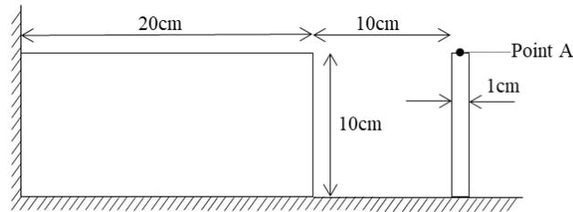
Figure 3 Granular flow simulations with an obstacle. Geometry
