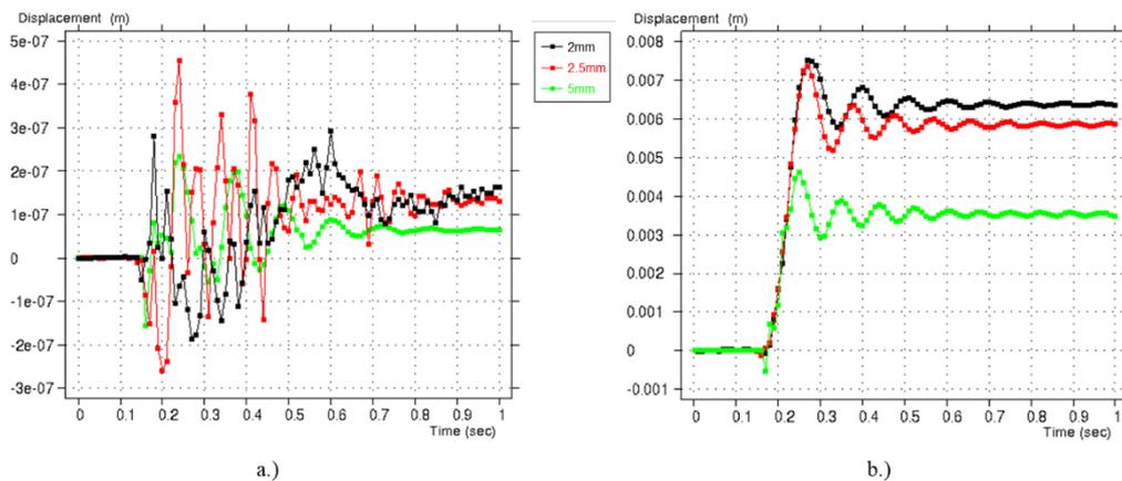
Figure 5 Displacement of (a) rigid and (b) flexible structure at point “A” upon impact and how it changes with respect to mesh refinement
