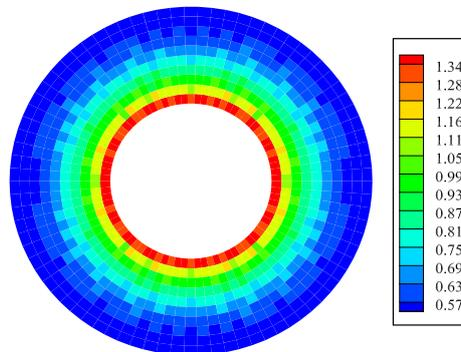
Figure 5 Contour plot of the circumferential stress for a linear-elastic cylinder subject to internal pressure
