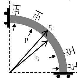
Figure 3 Sketch of a linear-elastic cylinder subject to an internal pressure
