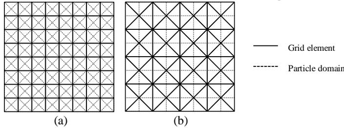
Figure 1 Initial discretization for the simulation of an axis-aligned displacement of a unit square using: (a) triangular particle domains with quadrilateral grid elements and (b) quadrilateral particle domains with triangular grid elements in a cross-patched configuration
