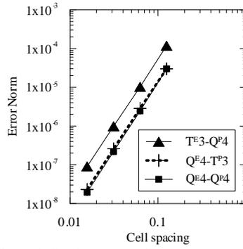
Figure 2 Convergence curves for the axis-aligned displacement in a unit square problem using CPDI2 with various particle domain and grid element shapes
