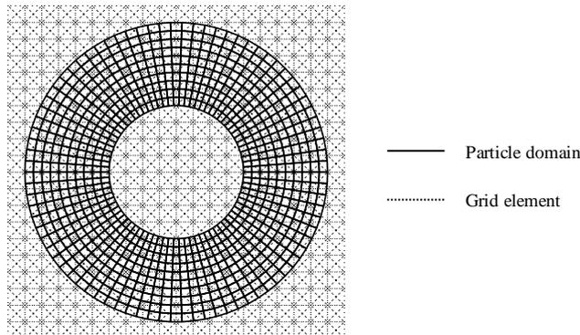
Figure 4 Discretization of a linear elastic cylinder using quadrilateral particle domains and triangular elements arranged in a cross-patched configuration
