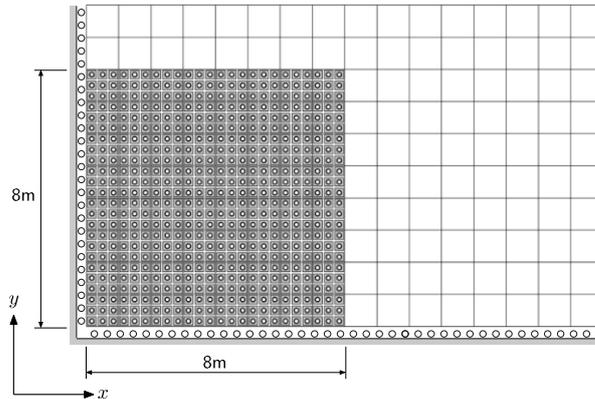
Figure 2 Elasto-plastic collapse: problem definition and initial discretisation
