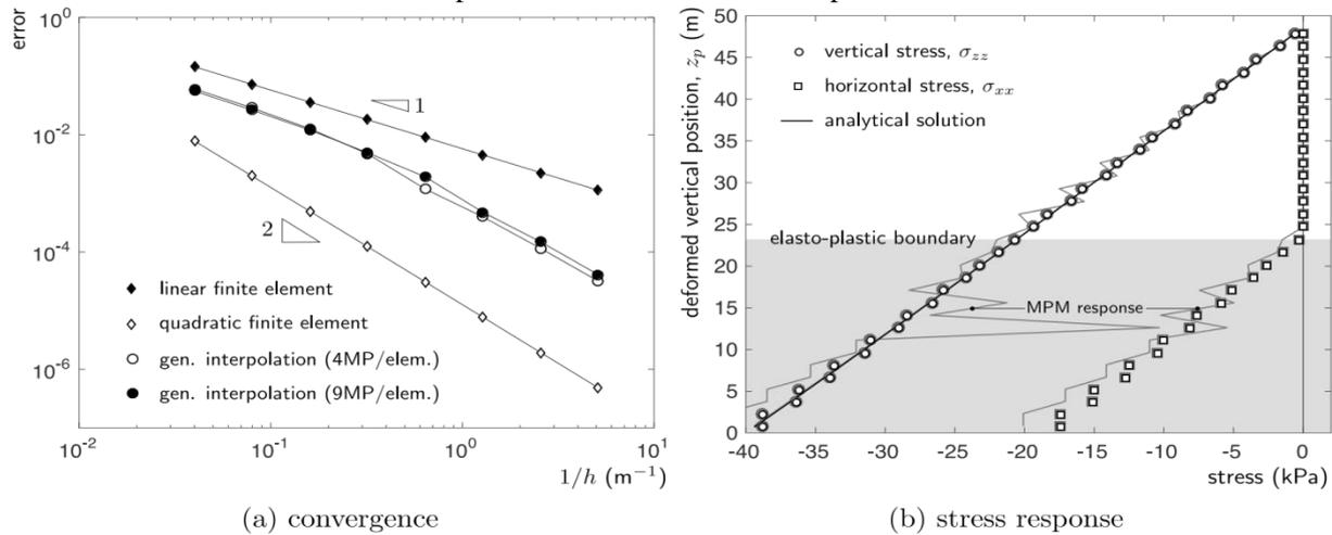
Figure 1 Elasto-plastic compaction under self weight
