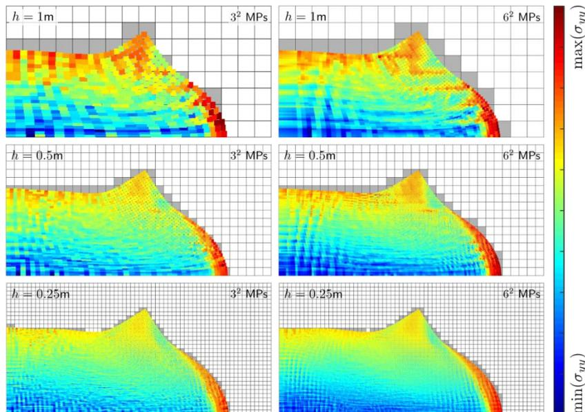
Figure 3 Elasto-plastic collapse: deformed material point positions coloured according to vertical normal Cauchy stress,  $\sigma_{yy}$ , where the mesh size,  $h$ , is given in each subfigure. The analysis was run with  $3^2$  and  $6^2$  material points per initially populated background grid cell
